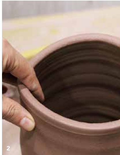
2 Use your fingers to square off the rim to create a four-sided form.
